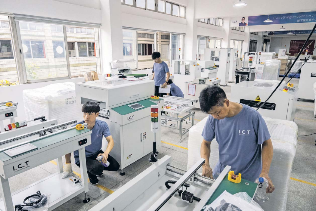
Employees on the job at China’s Dongguan ICT Technology, which makes automated systems that assemble circuit boards.
