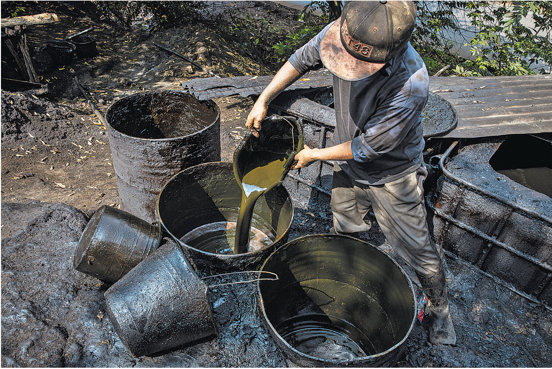
A worker pouring crude oil into a drum for heating and distillation. The crude will boil in a furnace to separate out water and then be sold as unrefined diesel.
